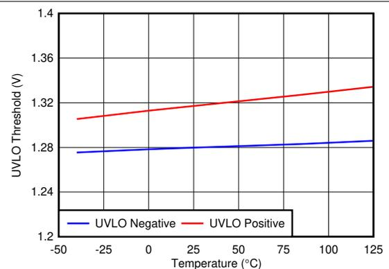
Figure 5-24. UVLO Threshold vs Temperature
