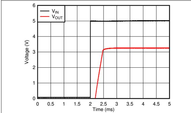
Figure 5-9.  $V_{IN} = V_{EN}$  Power-Up
