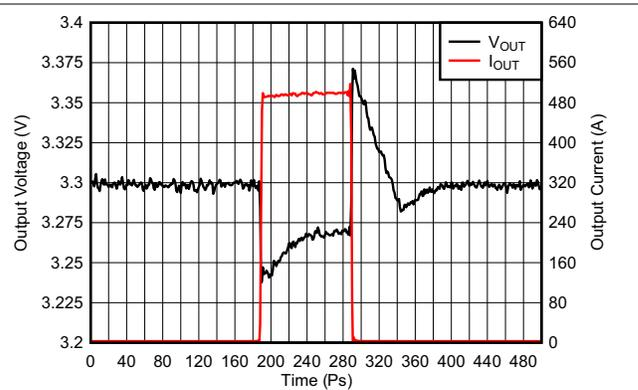
$V_{IN} = 5\text{ V}$ ,  $V_{OUT} = 3.3\text{ V}$ ,  $C_{OUT} = 1\text{ }\mu\text{F}$ ,  $I_{OUT}$  slew rate =  $1\text{ A}/\mu\text{s}$
