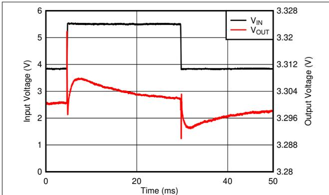
$V_{OUT} = 3.3\text{ V}$ ,  $C_{OUT} = 1\text{ }\mu\text{F}$ ,  $V_{IN}$  slew rate =  $1\text{ V}/\mu\text{s}$
