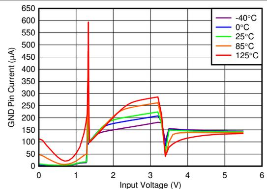
**Figure 5-18.  $I_{GND}$  vs  $V_{IN}$**
