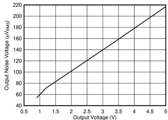
**Figure 5-6. Output Noise Voltage vs  $V_{OUT}$**
